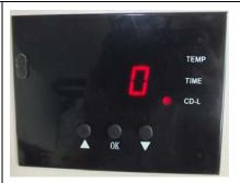
Press button after time setting; the display shows the temperature starts to rise. "CD-L" shows the time counting down during your transfer.
