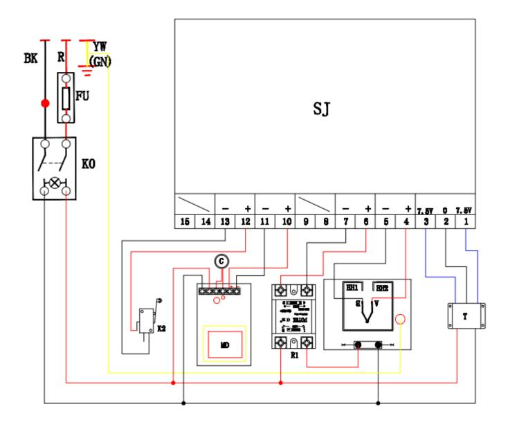
K<sub>0</sub>.: Power switch C: Magnet K2: Limit Switch
