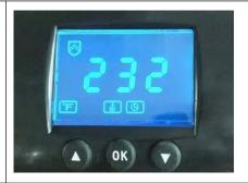
When you close the heat platen and start to transfer, the time starts to count down, once time is up, open the heat platen and start the next cycle.
