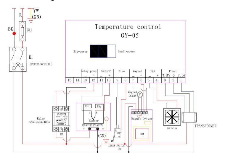
K<sub>0</sub>: Power Switch C:Magnet K2: Limit Switch
