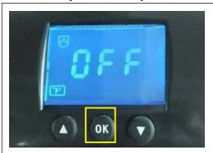
Turn on power switch, temperature light is ON. The digital display shows OFF
