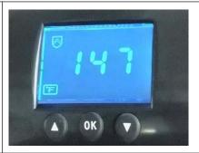
Press button after time setting; the display shows the temperature starts to rise. When the temperature rises to the setting temperature, the buzzer sends out sounds; then close down heat platen (meantime the sounds stop) and starts to transfer.
