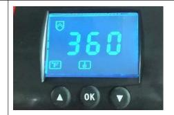
Press button, the temp light is on. Select with arrows the temperature according to different transfer material (such as 360°F).
