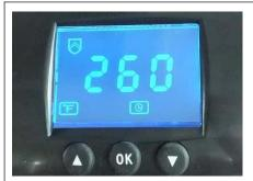
Press button after temperature setting and the itime light is on. Select with arrows the time according to different transfer material (such as 260s).
