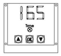
5. After finishing above-mentioned settings, press "OK" button to enter the heating mode. If the temperature is below 100C/212F, then the display reads "LO" (low temperature).
